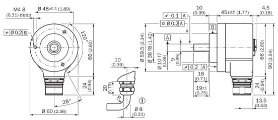
General tolerances according to DIN ISO 2768-mk ① R = min. bending radius 40 mm
