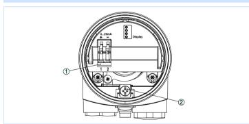
Electronics and connection compartment, single chamber housing
